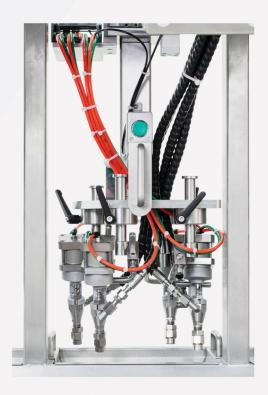
Our new improved paint filling machine can be used to fill paint and solvents. Change parts and paint are quick-changeable, with cleaning system in place. (CIP). The change of colour can be done in less than one minute.
