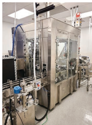
Tri-Pac Line 7 – MBC Aerosol Filling
